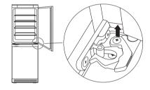
With the freezer compartment door closed, remove the crosshead screws from the lower door bearing and remove the door bearing downwards.
